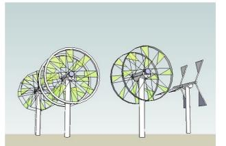
Fig. 12 Several types of wind systems taking advantages of rings and of double convergent turbines.
