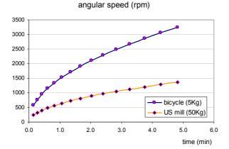
**Fig. 5** Ideal angular speed responses for a bicycle wheel of 5Kg, 2 m radius, and an equivalent American windmill of 50Kg, when receiving a constant power of 8 KWatt, with efficiency of 50%.
