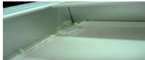
Figure 7: Non uniform sealant in the back sheet. It can produce inclusion of moisture and dielectric problems.
