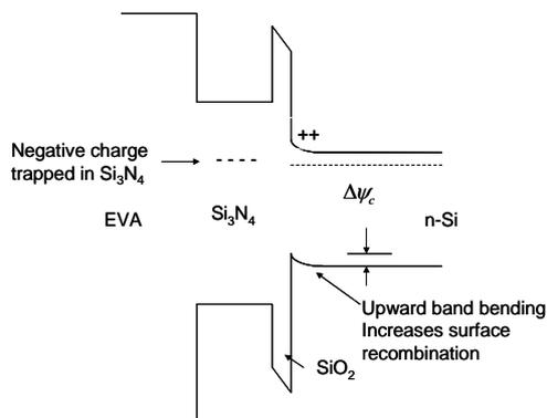
**Figure 3:** Band structure at the front surface of a back-contact cell.
