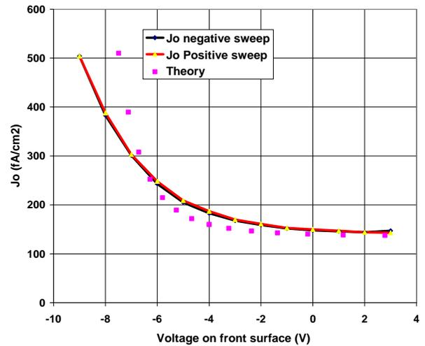
**Figure 4:** Measured and theoretical cell saturation current as a function of voltage applied across the front passivation oxide.
