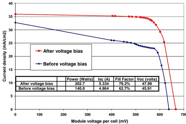
**Figure 5:** Module performance after receipt from the field and after voltage bias.
