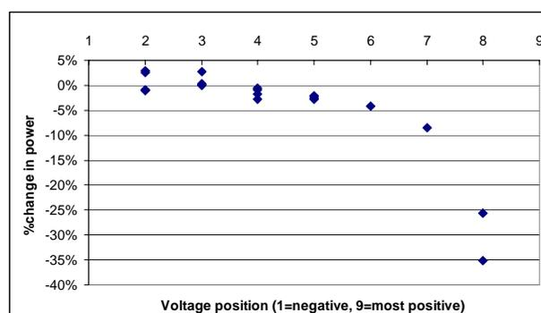
**Figure 1:** Change in power versus module position in several series connected strings after several months of outdoor operation.
