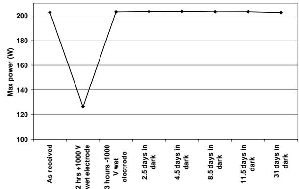
**Figure 7:** Example of a module which was polarized at 1000 V, then recovered at -1000 V, after output remained constant.
