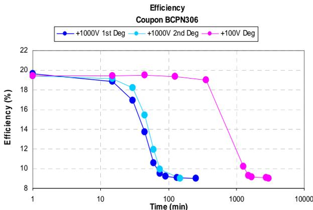
**Figure 6:** Voltage dependence of output reduction due to front surface polarization.
