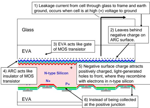
**Figure 2:** Cross-section of a back-contact solar cell embedded in a module showing the top, n-type passivation layer capped with a silicon dioxide, silicon nitride ARC layer[1].
