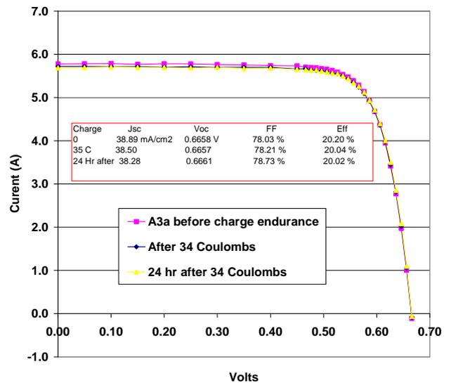
**Figure 8:** Cell IV curves before and after passing 34 coulombs through the front passivation. No change in performance is seen.
