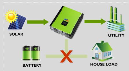
In this operation mode, the inverter will only behave like a pure grid-tie inverter where it only feeds back electricity to grid from PV source.
