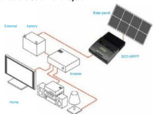
Combined MPPT technology and DSP controller, SCC-MPPT will convert best voltage to charge battery based on varied temperature. Compared to traditional solar charge controller, it allows your solar panels to operate at their optimum power output voltage, providing higher efficiency up to 98% with lower power loss.
