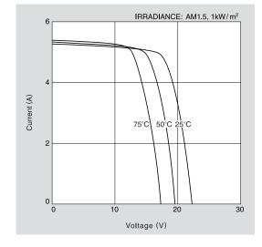
Current-Voltage characteristics of Photovoltaic Module KC85T-1 at various irradiance levels
