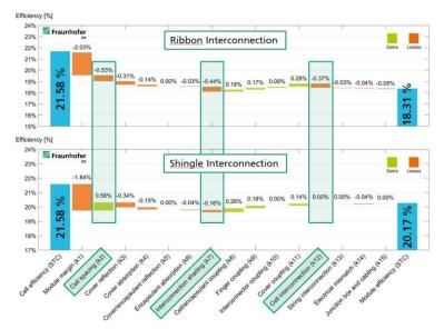
Screen shot of a waterfall diagram from the software package SmartCalc.CTM of Fraunhofer ISE, where the efficiency gains and losses of a shingle cell module to a module with conventional cell interconnections are compared. ©Fraunhofer ISE
